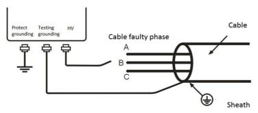
Phase-phase fault wiring as below:
