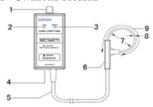
Output Interface: standard BNC interface, connect to any manufacturer oscilloscope with the BNC Cable.
