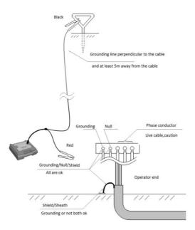
Fig.3.8 Null / Ground / Shield Injection Method
