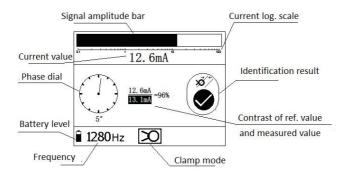
Fig.5.2 Clamp identification interface
