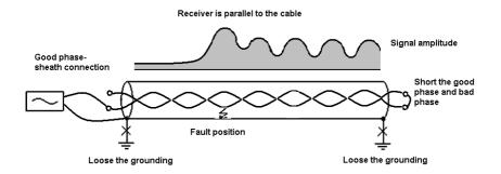
Fig.7.2 Phase to armor grounded fault pinpointing
