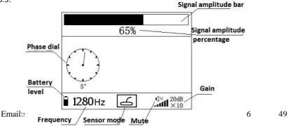
Fig.5.5 Sensor identification mode interface
