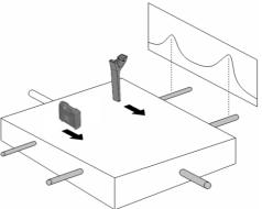
move simultaneously at the direction perpendicular to the cable/pipe. When the Transmitter passes the cable/pipe, the signal will be inducted into the pipe and the Receiver will receive signal. Observe the receiver responding and mark on the ground when peak responding above the pipe. Refer Fig. 4.8
