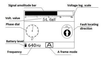
Fig.6.3 Interface for A frame fault location
