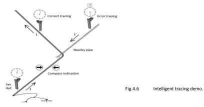
The process of Correct/Error indication as below Fig. 4.6
