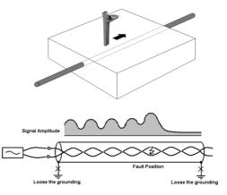
connection output mode, and should connect to two fault core wires. <u>The receiver must</u> be moving parallel to the cable, and use the peak method to detect.
