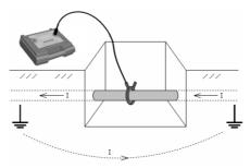
Fig.2.7 Clamp coupling mode wiring
