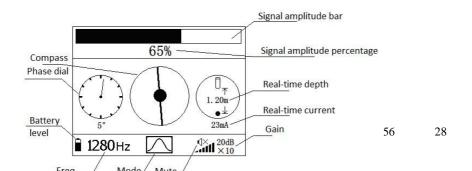
Fig.4.1 Pipe detection interface diagram
