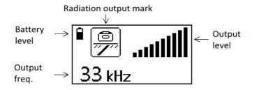
Fig.2.10 Radiation mode measurement diagram
