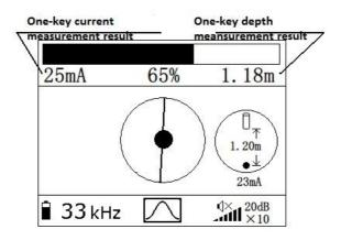
Fig.4.12 One-key depth and current measurement
