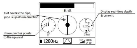
Fig.4.11 Real-time depth and current measurement
