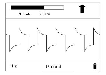
The arrow in the pic. is the current direction. Before fault point, the arrow is upward. If loop ground, arrow is downward when behind the fault point. In the upper part of screen, there will be the current value display and meanwhile show the current waveform. If system has ground, the screen bottom will have Ground indicating and audio alarm.
