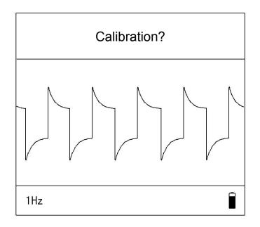
When screen display Calibration? Press CALI. button to calibrate after the waveform stabilization.
