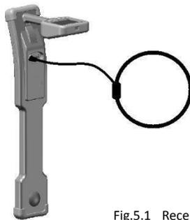
Fig.5.1 Receiving clamp connection
