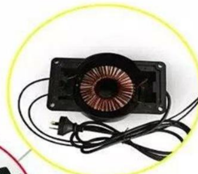
2. Before potting epoxy resin
