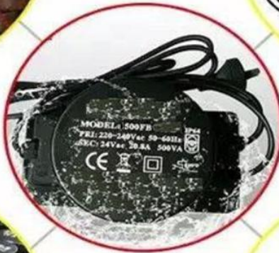
2. Before potting epoxy resin
